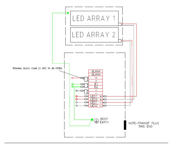
Note: For 24 LED luminaires, there will only be one LED array connected to the terminal block.
